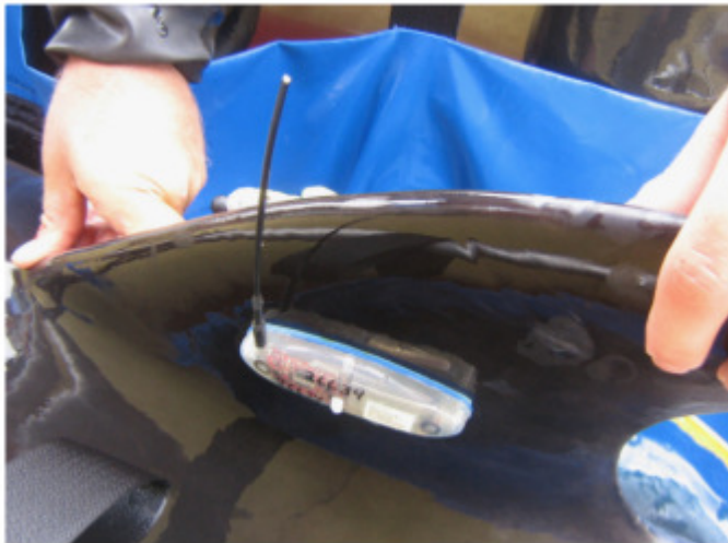
Fig. 2. A satellite tag (SPOTS, Wildlife Computers, WA, USA) was attached to the dorsal fin of the male dolphin.
